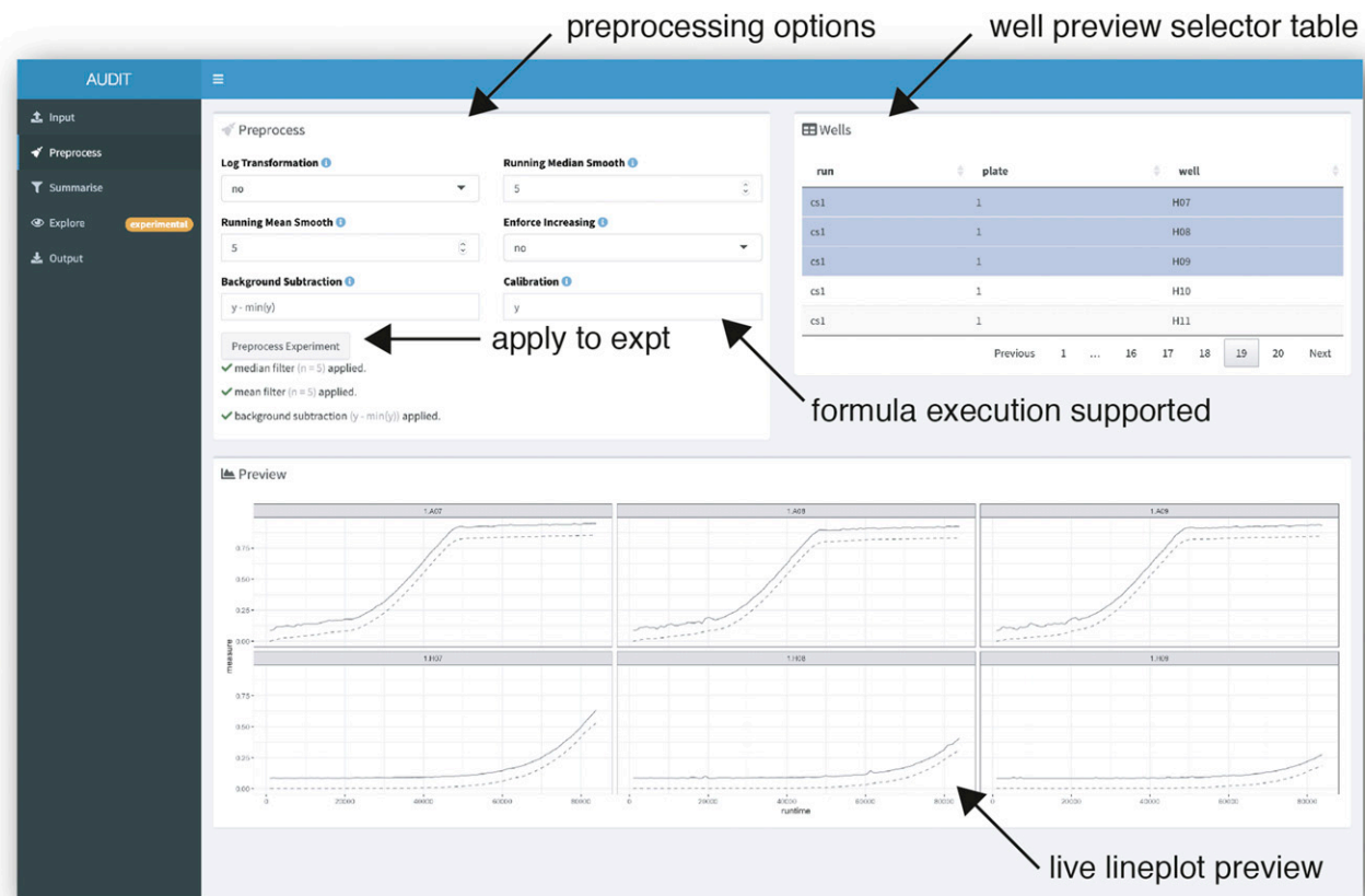
Figure 4 Live preview and flexible specification of varied preprocessing methods. Screenshot of preprocess panel. AUDIT makes six independent preprocessing options available (arrow, top-left). The Background Subtraction and Calibration input fields support arbitrary formula (code) execution (arrow, middle-right). The well preview selector table (arrow, top-right) contains data from selected runs in the experiment. When clicked, the 'Preprocess Experiment' button applies the preprocessing to the whole experiment (arrow, middle-left). To display a live plot preview, users select rows in the table. Then, AUDIT plots each well's raw (solid line) and preprocessed measures (dashed line) (arrow, bottom-right).
