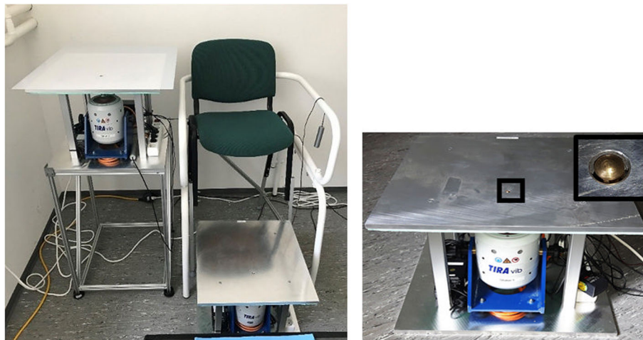
Fig. 7 Left: Vibration perception threshold set-up for measuring hand and foot sensitivity. Right: Platform with tip of vibrating probe (black squares)
