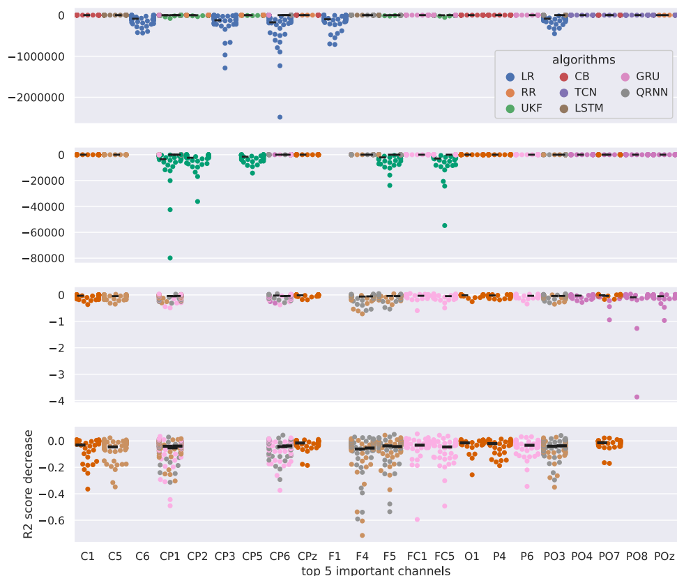
Figure 11. Feature of importance in channel assessment for each decoding algorithm evaluated with R2 score. There are four plots that share the same x-axis with the channel of importance after input perturbation analysis. The y-axis shows the decrease in the R2 score after the perturbation of the channel. The first plot includes all the decoding algorithms. The second plot shows algorithms without LR and RR. The third plot shows the algorithms without LR, RR, and UKF. The fourth plot shows algorithms without LR, RR, UKF, and TCN. The thick black line represents the median decrease in R2 score for each algorithm for each channel.
