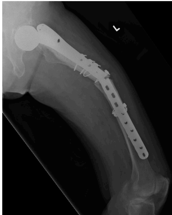
Fig. 16. Radiograph (lateral view) showing breakage of the locking plate with fracture displacement.
