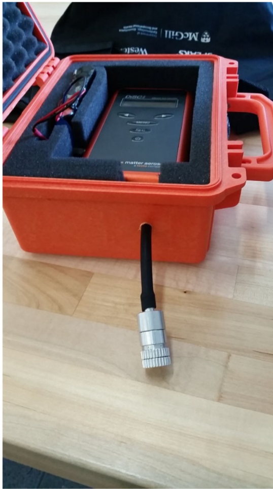
Figure 2: Left: DiSCmini instrument used to measure ultrafine particle number concentration. Right: Example set-up of DiSCMini and pDR monitors.
