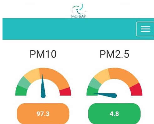
Figure 8. Chart representing the concentrations of PM 10 and PM 2.5 in µg/m 3 as shown by the mobile app.
