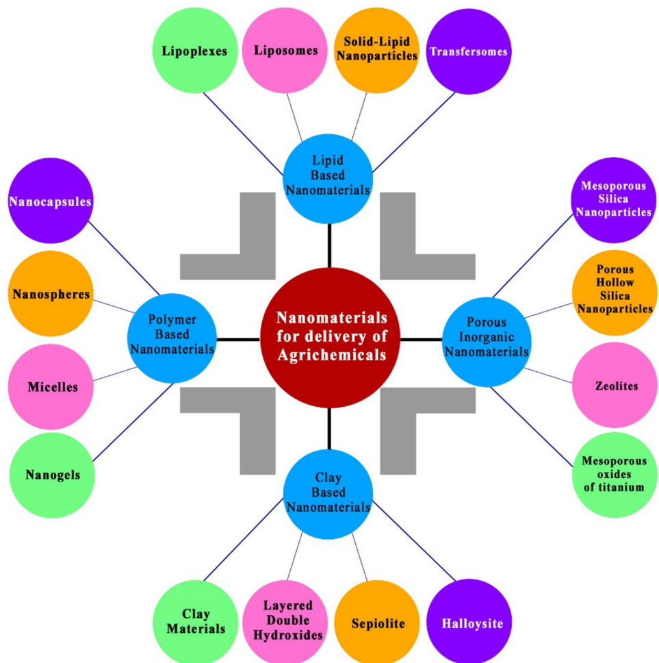
Fig. 2 The lipid, polymer, clay and porous inorganic-based nanomaterials for the delivery of agrichemicals (nanopesticides and nanofertilizers) to the plants through application in soil
