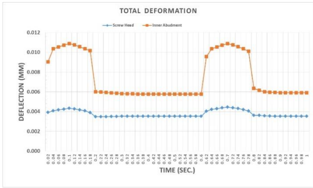
Figure 10. Comparison of the maximum displacement of the screw head and the internal part of the octagon abutment at their interface during preloading and vertical loading.
