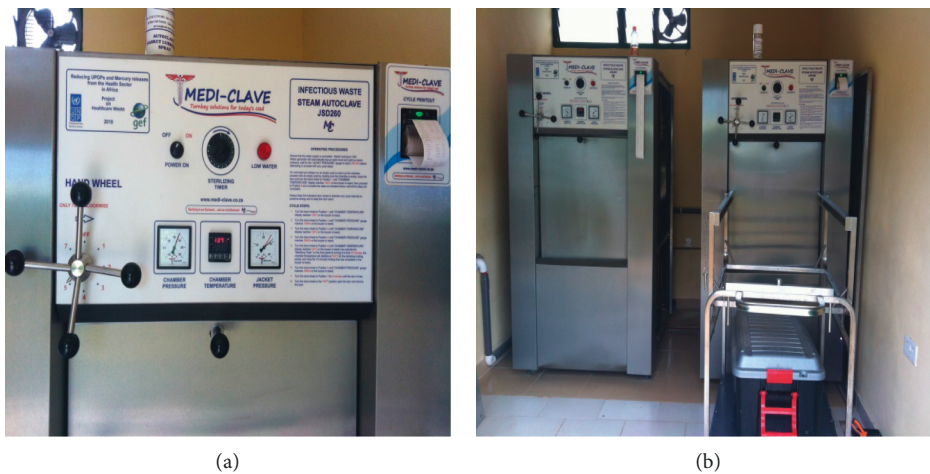
FIGURE 12: Central autoclaves for infectious waste sterilization at the CCTH, Cape Coast, Ghana.
