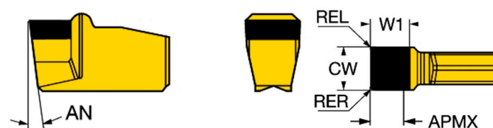
Figure 2. T-Max ® Q-Cut insert for grooving (N151.2-600-50E-G CB20) [11].
