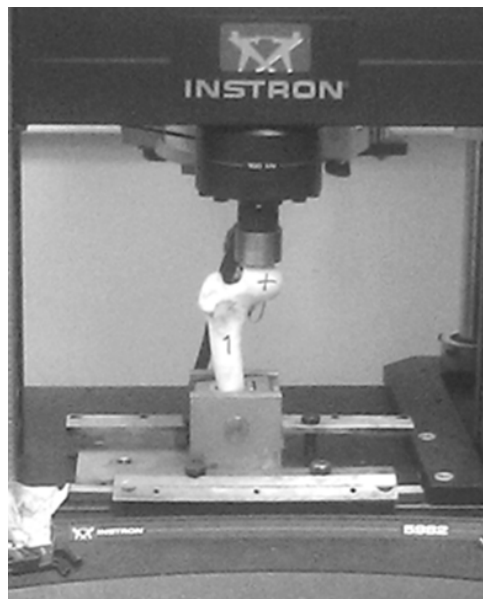
Figure 11. Testing procedure of the reinforced hip sample.
