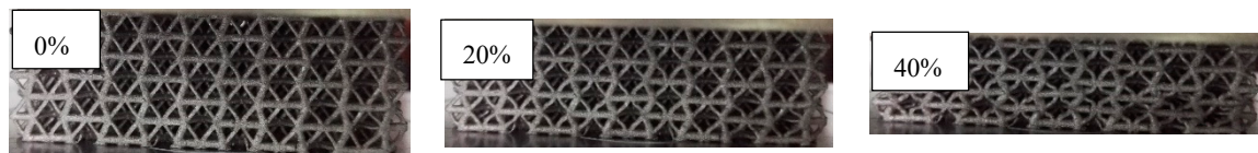
Figure 5. The deformation modes of the structure at different strain regions.
