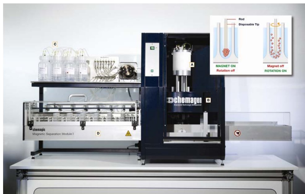
Fig. 2 chemagic Magnetic Separation Module I consisting of (A) separation head with magnetizable rods [here 12-well format for large (50 ml) volumes; 96-well format for MTPs also available], (B) electro magnet, (C) chemagic dispenser for parallel filling of all required buffer solutions (accessory) and (D) tracking unit. The principle functionality regarding separation and resuspension of magnetic beads is shown in the scheme
