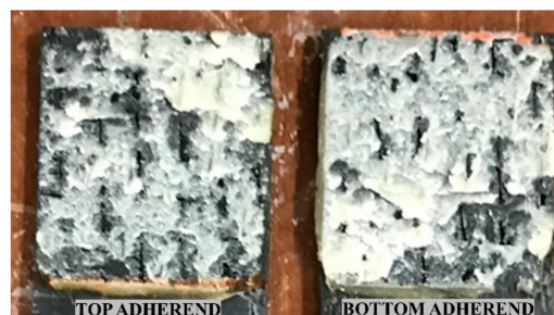
Figure 10. Failure surfaces of adhesively bonded ELC_ELC composites.
