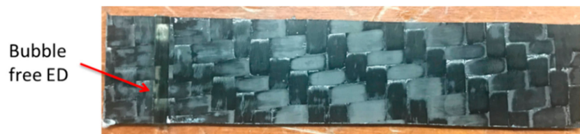
Figure 4. Manufactured Energy Director (ED) laminate with optimized parameters.
