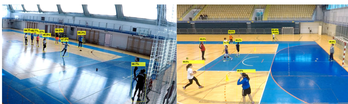
Figure 3. Bounding boxes with confidence values as results of person detection with YOLOv3.
