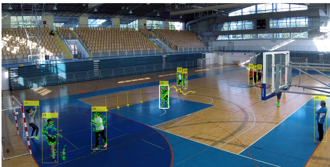
Figure 8. Detected most active player (white thick bounding box) and his trajectory through the whole sequence (yellow line).
