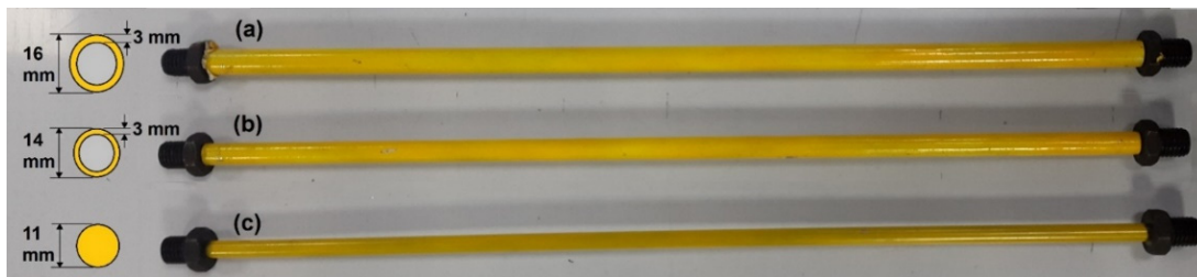
Figure 4. Details of the damaged elements with; (a) 20%, (b) 50%, and (c) 80% reduced percentages of the cross-section stiffness.
