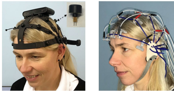
Figure 1. EEG headsets. Left: Dry and wireless EEG system: F1 headset with Ag electrodes. The module on top of the headset contains all units to process, store and transmit the EEG signals. The insert shows the dry electrode as mounted at each of the 19 10–20 electrode sites. Right: Wet and wired EEG system: Inomed recording net with Ag/AgCl electrodes.
