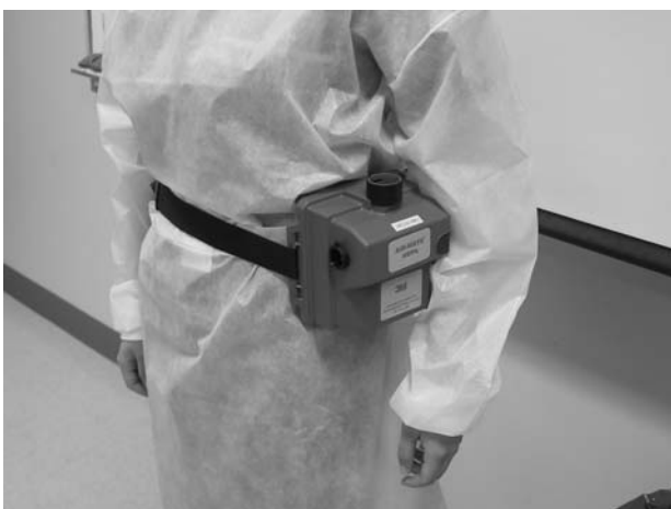
FIGURE 2 The powered air-purifying respirator (PAPR) system consists of a belt-mounted powered air purifier with a high efficiency particulate air (HEPA) filter.
