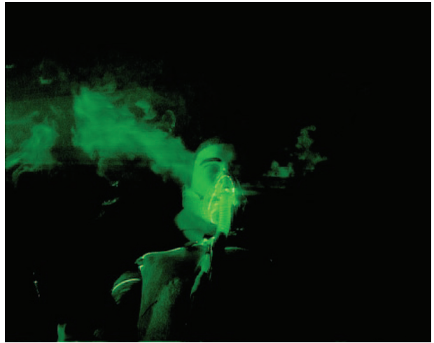
FIGURE 1. A simple oxygen mask attached to a high-fidelity HPS with a laser light-sheet on the right side. The simulator represented a 70-kg adult male sitting on a hospital bed inclined to 45° and was programmed to breathe spontaneously. The lung compliance was set as 35 mL/cm H 2 O, and the oxygen consumption to 350 mL/min. Tidal volume and respiratory rate were regulated so that a respiratory exchange ratio of 0.8 was maintained during measurements. Typically, this was achieved with a tidal volume of 500 mL at a rate of 14 breaths/min. These conditions represent a patient with mild lung injury.
