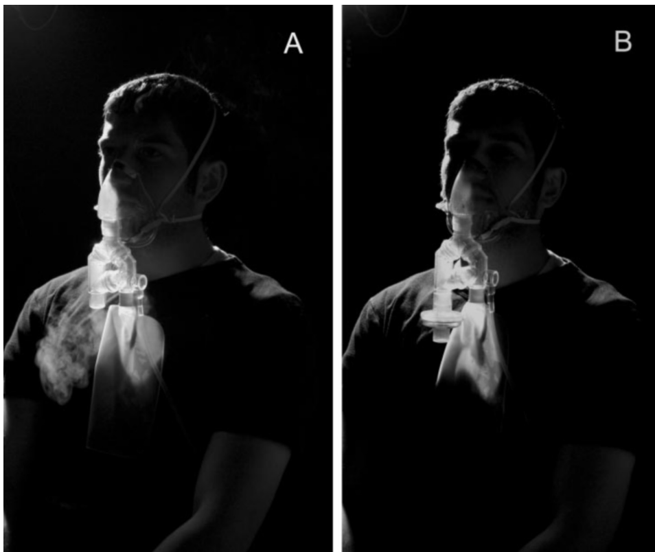
FIGURE 2. Subject exhaling previously inhaled saline aerosol mist while wearing Hi-Ox80 oxygen mask without an added filter placed on the exhalation port ( left, A ) and with added filter placed on exhalation port ( right, B ).
