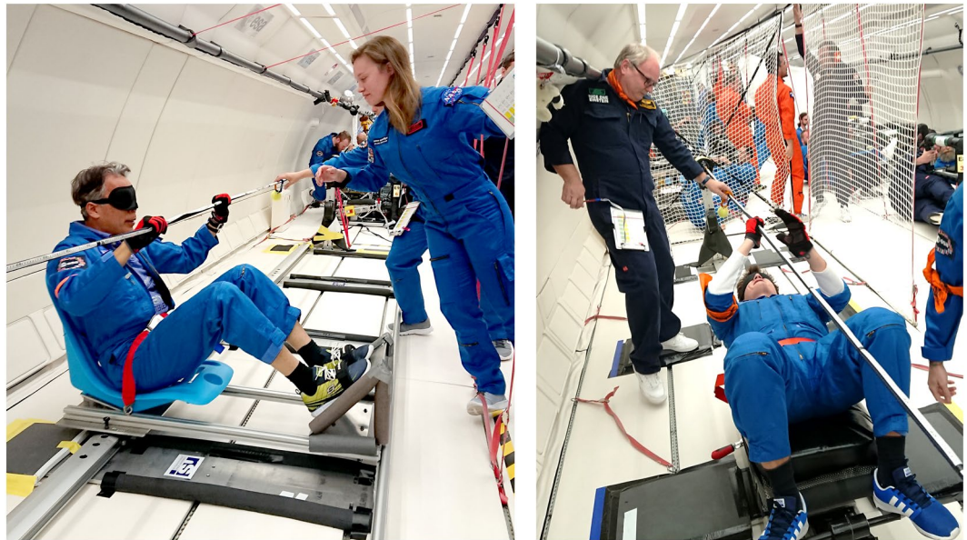
Figure 1. Experimental set-up for measuring lateral (left) and vertical (right) distance judgments. Subjects were either sitting upright and moving to their right/left or lying on their back and moving up/down by pulling on a rope. Photos courtesy of Novespace.
