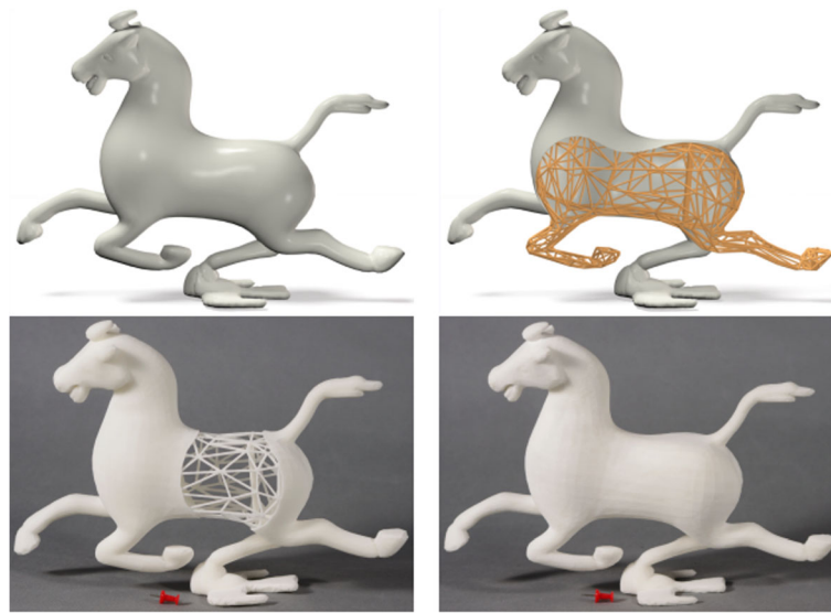
Fig. 1 Skin-Frame lightweight structure design and manufacturing results by 3D printing [16]
