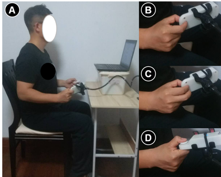
Fig. 1 The standardized positioning (a) used for tip (b), palmar (c), and key pinch (d) force sense measurement
