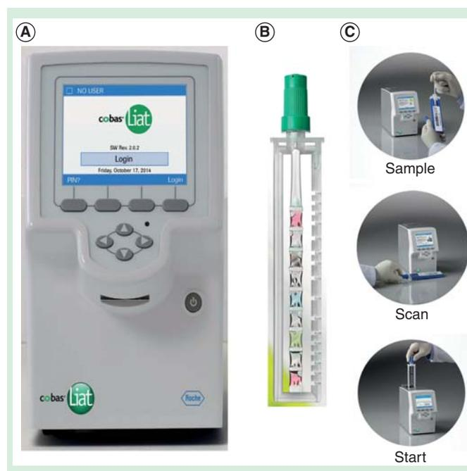
**Figure 3. The Roche Diagnostics cobas Liat. (A)** Instrument; **(B)** PCR-based sample processor; **(C)** Workflow. Figures provided courtesy and permission of Knowledge Optimization<sup>®</sup>, Davis, California, and Visual Logistics.
