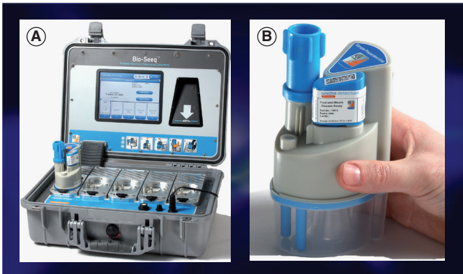
Figure 4. BioSeq Portable Veterinary Diagnostic System. (A) Portable PCR instrument with five independent thermocyclers (running assay in far left thermocycler) with built in communications, including global positioning system, WiFi and Bluetooth technology. (B) Disposable automated sample-preparation unit processes raw sample into PCR mixture allowing test to be conducted at pen-side.
