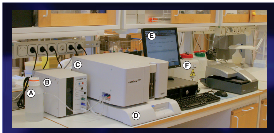
Figure 2. Luminex laboratory at the National Veterinary Institute and the Swedish University of Agricultural Sciences in Uppsala, Sweden. Luminex 200™ system, including (A) waste bottle, (B) the Luminex SD sheath fluid-delivery system the (C) Luminex 200 instrument, the (D) Luminex XY plate-handling platform and (E) Luminex xPONENT 3.0 software and a PC. The microsphere-based detection system allows for 100 different analytes to be detected in each sample (100-plex). Also pictured, is (F) the Tecan Hydroflex wash-station with buffer and waste bottles. This instrument performs automated microplate washing and vacuum filtration for use with both bead types (magnetic and polystyrene) used in the Luminex system.
