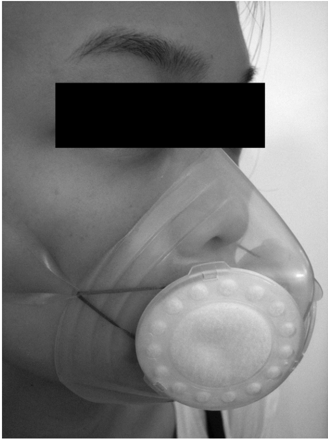
Figure 1. Totobobo mask. Inspired gas is filtered by high-efficiency particulate air (HEPA) filters. Plastic can be cut to fit the wearer's face. Transparency allows observation of contact between the plastic and the wearer's face.
