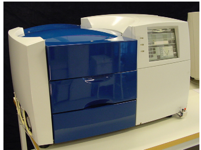
Fig. 4. QuanTyper instrument for performing ultra rapid PCR and sequencing (Alpha Helix). Features of the instrument: (a) high speed and sensitivity: 100 \mu L real time Q-PCR in <11 min; (b) cycle sequencing reaction: 500 bases in <15 min; (c) high convenience in combination with Capillette. Sample volume ranges 20–200 \mu L.
