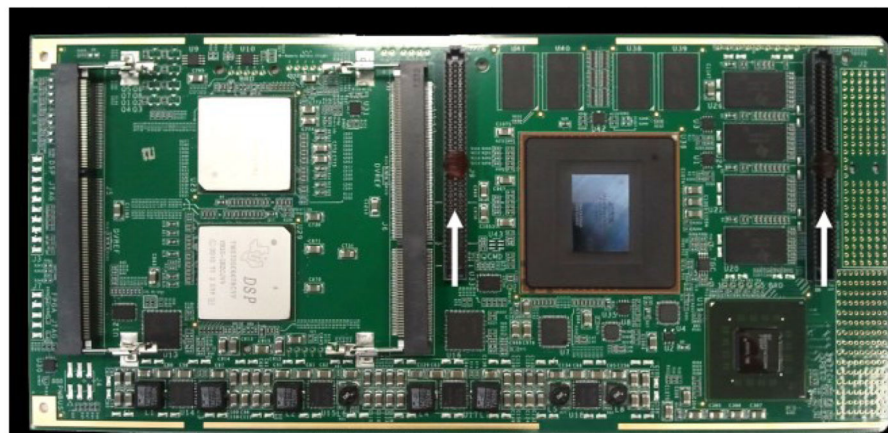
Fig. 2. The Front-End board. Top: Block-diagram; Bottom: view of the upper board side showing the FPGA (on the right) and the two DSPs. The high power TX and T/R switch board is hosted by the high-speed connectors indicated by white arrows.
