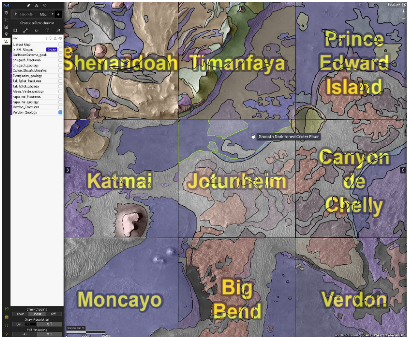
Fig. 4. The CAMP tool developed by Calef and Soliman (2019) and used by the Mars 2020 Science Team to construct the photogeologic map. 1.2 by 1.2 km quadrangles were displayed in CAMP and assigned to individual team members who mapped units within the tool. Mapped geologic units shown are the raw, uncorrelated boundaries by mapping quad
