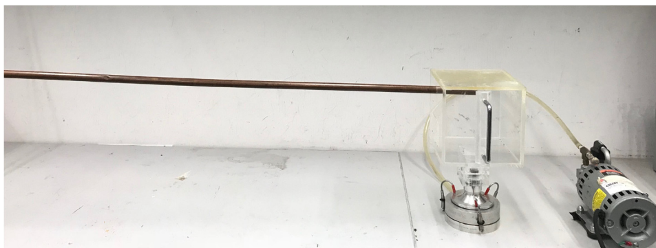
Fig. 4. A schematic of the copper tube-acrylic box sampling manifold.
