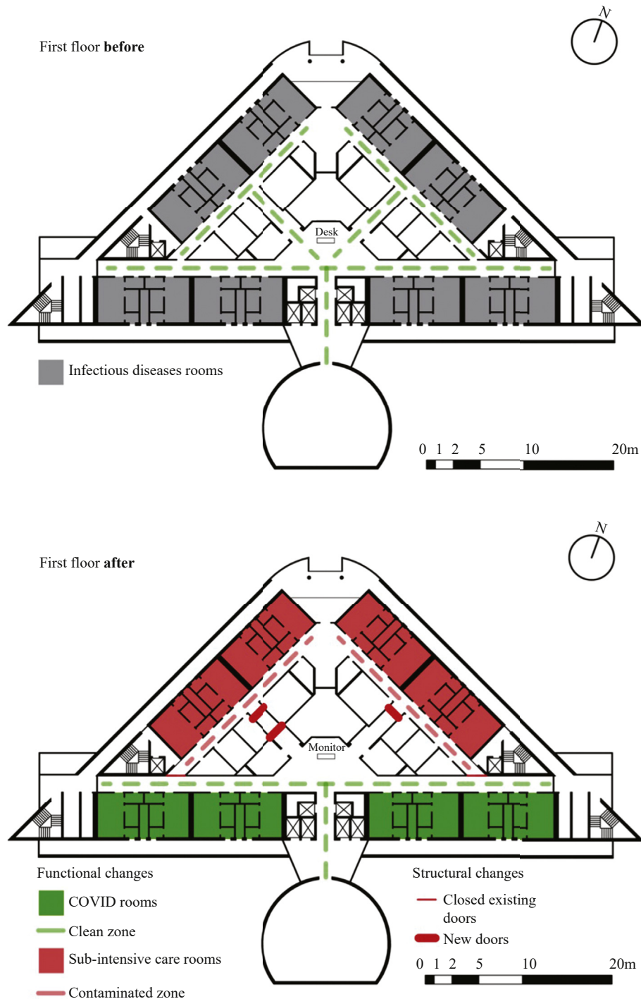
Figure 1. Layout of the first-floor Infectious Diseases ward before and after changes to accommodate the COVID-19 epidemic.
