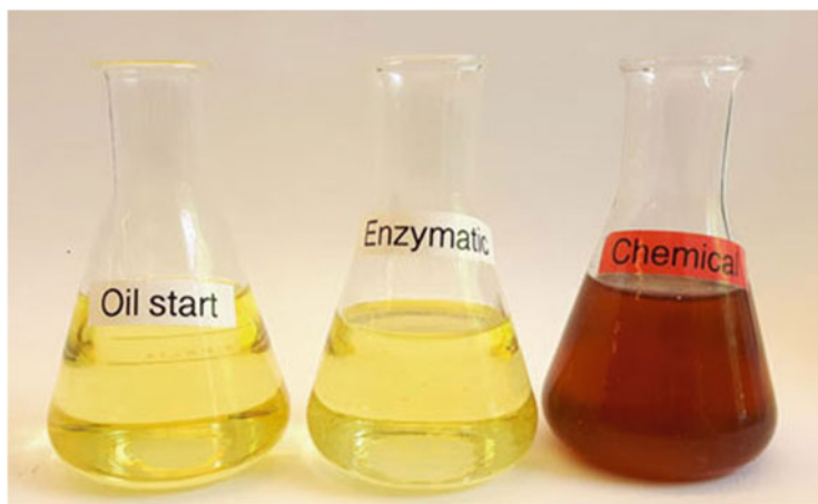
Fig. 7.2 Color change and by-product formation using chemical esterification (“Chemical,” right flask) compared to the use of a lipase (Lipozyme TL ® , a lipase from T. lanuginosus manufactured in A. oryzae ; “Enzymatic,” middle flask) using plant oil (“Oil start,” left flask)
