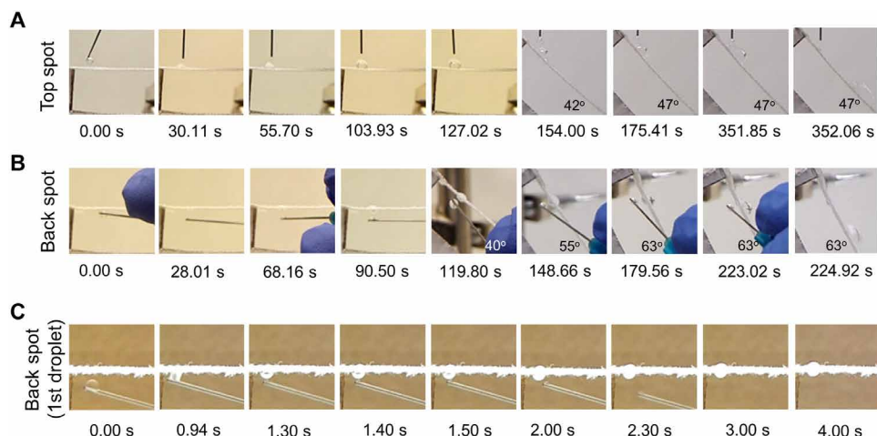
Fig. 4. Directional transport property and repellency of artificial sweat liquid on the superhydrophobic finished fabric after selective plasma treatment. (A and B) Still frames taken from videos when sweat droplet was dripped onto (A) exposed top spot and (B) unexposed back spot areas under a flow rate of 10 \mu\text{l}/\text{min} . The fabrics were originally laid horizontally and then were rotated clockwise to certain inclined angles. The back spot was tested via dripping sweat liquid initially upward against the gravity. (C) Transport behavior of a first sweat droplet when being dripped upward to the back spot of the horizontally laid fabric. Movie credit: Lihong Lao, Cornell University.
