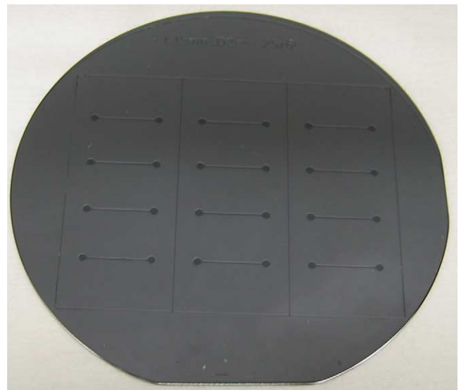
Fig. 2. Picture of the PDMS master molding whose microfluidic flow channels were fabricated using SU-8/25. Each channel was 15,000 \mu\text{m} in length, 500 \mu\text{m} in width and either 50, 18 or 8 \mu\text{m} in height.
