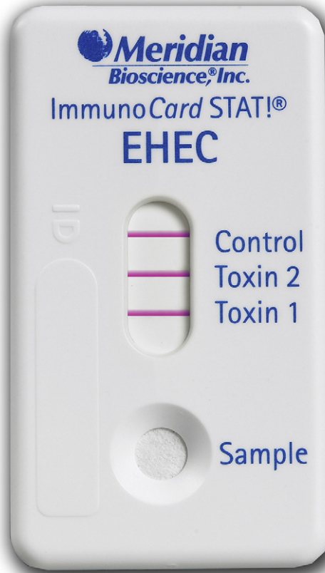
Fig. 5. Shiga toxin lateral-flow immunoassay device for testing broth and agar cultures. This device distinguishes Stx1 from Stx2. (Courtesy of Meridian Bioscience, Cincinnati, OH.)
