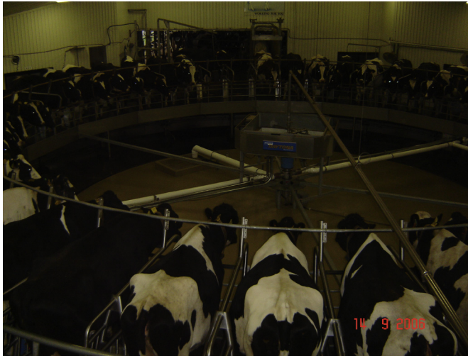
Fig. 5. View of Great Hopes' fully loaded 50 stall rotary parlour from an observation room. Cattle enter at 12:00 o'clock and exit by backing out of the apparatus at 11:00 o'clock. (Photograph taken by the author).
