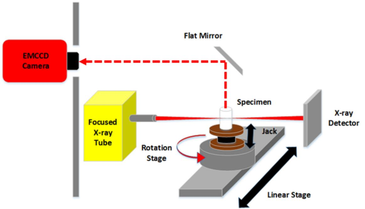
Fig 1. Schematic of the experimental XLI set-up.
