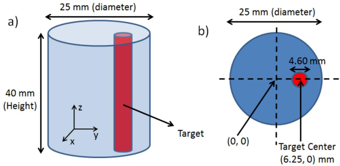
**Fig. 3.** Phantom geometry for the XLI experiment. a) overall phantom geometry and b) top surface geometry showing target location. Note: The GOS:Eu<sup>3+</sup> target is for the 3rd phantom only.
