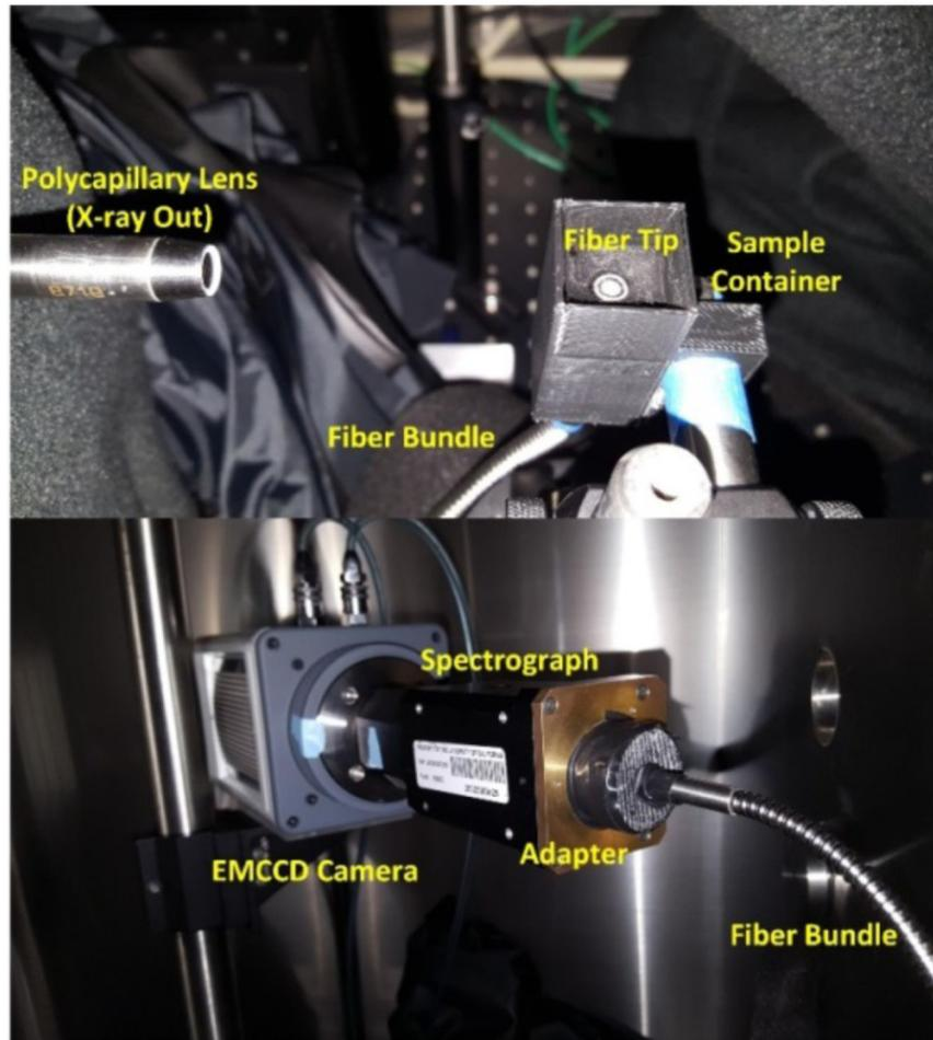
**Fig. 6.** Photograph of the x-ray luminescence spectra measurement set-up. The sample container is shown without the cap so the fiber tip can be visible in the photo. The bottom photo shows the other end of the fiber which delivers the emitted photons to the spectrograph and the EMCCD camera.
