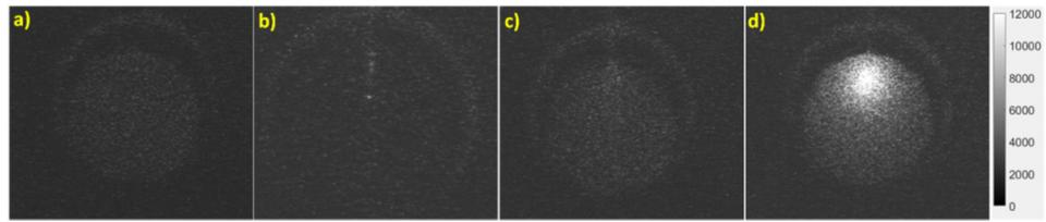
**Fig. 7.** Top surface EMCCD camera images for the 5 mm scan depth. a) background image (x-ray off), b) agar phantom (x-ray on), c)  $\text{TiO}_2$  phantom (x-ray on), d)  $\text{GOS:Eu}^{3+}$  phantom (x-ray on). The grayscale indicates the luminescence intensity in arbitrary units.
