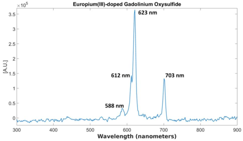
**Fig. 11.** Measured x-ray luminescence spectrum for GOS:Eu<sup>3+</sup> particles.
