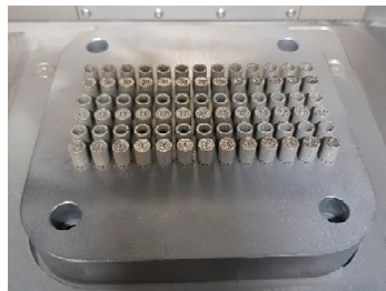
Figure 6. Samples for the static and dynamic compressive tests on the SLM 125 HL machine building platform.
