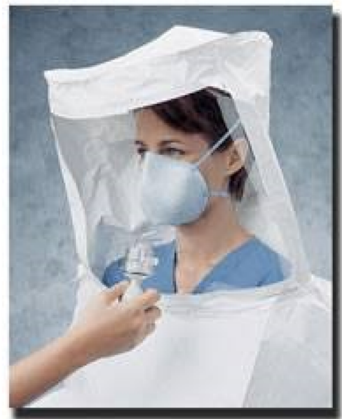
Fig. 4a. fit testing N95 mask with qualitative solutions (isoamyl acetate, saccharine, etc.).
