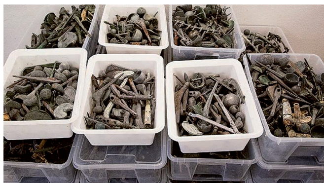
Retrieved metal implants after cremation sent for recycling. (With permission from Jennie Lorentsson).
