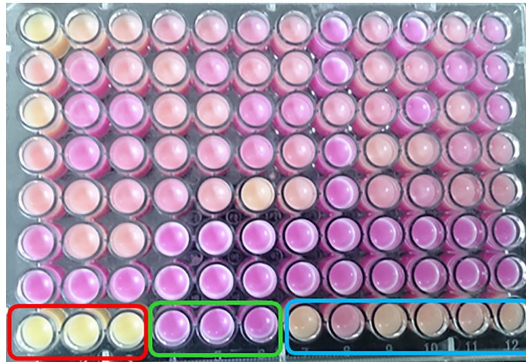
Fig 4. Change of pH due to hydrolysis of triglyceride by mutants of GTL indicated by phenol red. Wells in red rectangle are positive controls (pH <6, without lipase), in green rectangle are negative controls (pH 9.5, without any lipase) and in blue rectangle are with GTL. Acidic samples are yellow in colour (due to activity of lipase) and alkaline samples are purple in colour.
