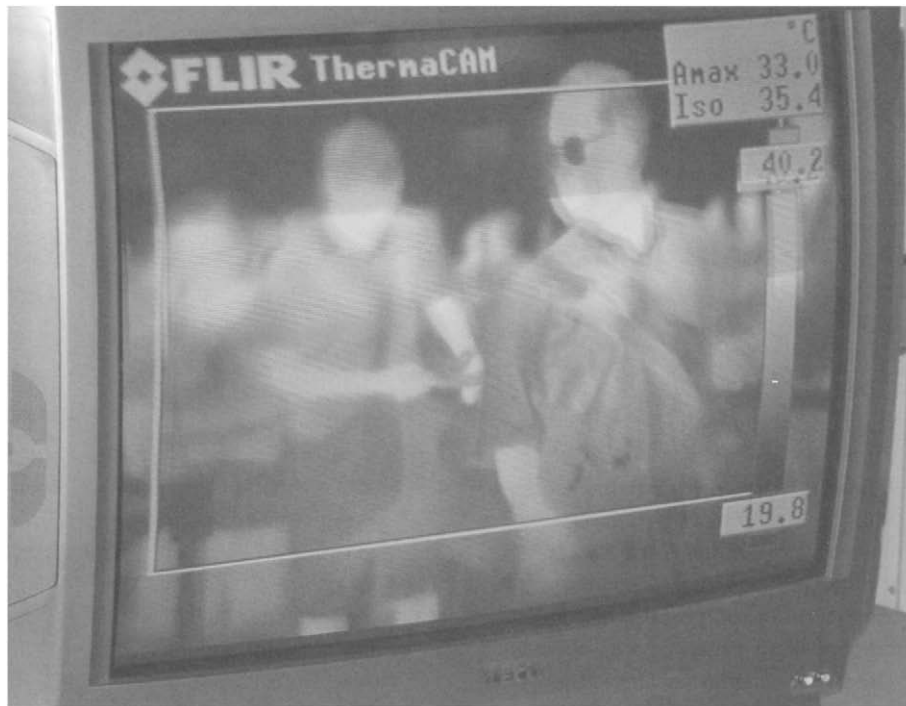
FIGURE 3.5 Thermal screening device at the Chiang Kai-shek Airport, Taipei. Lighter shades of grey correspond to higher temperatures (From Wagner.)
