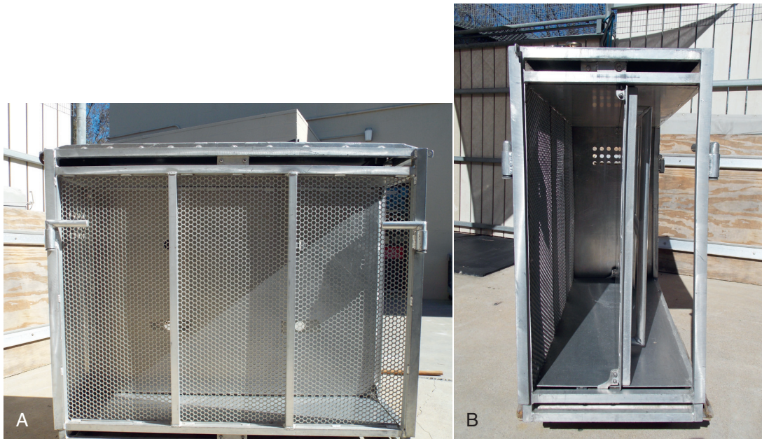
FIGURE 58-2 A , Metal squeeze chute or crate used for anesthetic induction of small- to medium-sized suids and peccaries. B , End-on view illustrating squeeze mechanism.
