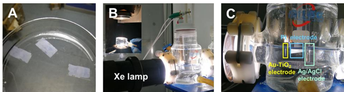
Figure S13. The photocurrent test related to Figure 4 . (A) The test apparatus. (B) The measurement of simulated sunlight intensity from the Xenon lamp. (C) The three-electrode system.
