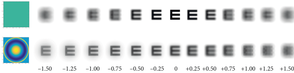
FIGURE 3: Illustration of the phase pattern and through-focus theoretical simulations of the Snellen E-letter of 30 arc-min for 4 mm pupil diameter (from -1.5 to +1.5 ). Top: diffraction-limited eye; bottom: aspheric-based design (spherical aberration: +0.25 \mu\text{m} ).
