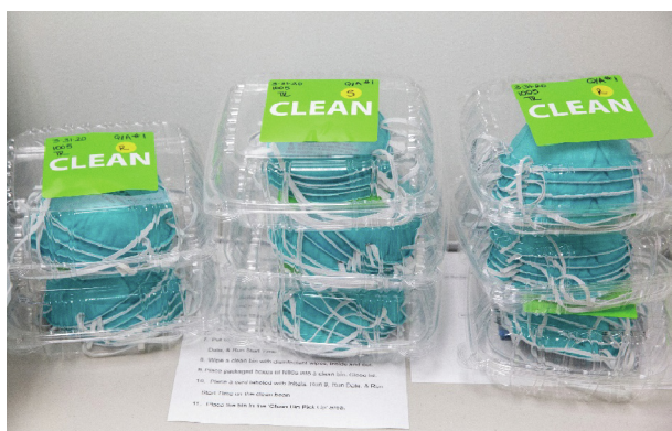
Fig. 1. N95 masks, like the “CLEAN” ones shown here, are being reused at Duke University Hospitals (Durham, NC, USA) after decontamination using a Bioquell (Horsham, PA, USA) Z-2 device (see Fig. 2) that uses hydrogen peroxide vapor for sterilization [1]. Credit: Duke University, with permission.
