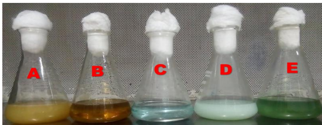
Figure 1. Observation of the color change in the reaction mixture of Pseudomonas fluorescens MAL2 during the biosynthesis of CuNPs: (A) P. fluorescens MAL2 in F-Base medium. (B) Cell-free extract supernatant. (C) \text{CuSO}_4 \cdot 5\text{H}_2\text{O} solution. (D) One gram of cell pellet added to \text{CuSO}_4 \cdot 5\text{H}_2\text{O} . (E) Color change in the reaction mixture from blue to dark green indicating the formation of CuNPs.
