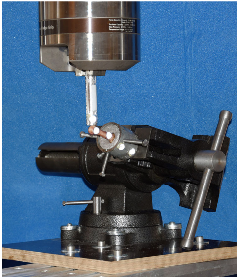
Figure 2. Biomechanical test setup. The potted fifth metatarsal specimen was fixed into a machine vice on an adjustable platform. A metal rod attached to the loading frame was used for force transmission in a plantar to dorsal direction. Light-reflecting hemispherical markers were glued onto the distal part of the Jones fracture specimen and onto the pot and rod for kinematic tracking. [Color figure can be viewed at wileyonlinelibrary.com ]
