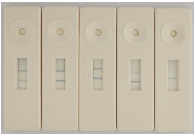
Figure 2 Sensitivity of the lateral flow device, tested with Xanthomonas campestris pv. musacearum NCPPB2251. Bacterial culture serially diluted in banana sap/buffer A from 10^8 cells \text{mL}^{-1} (left) to 10^4 cells \text{mL}^{-1} (right).
