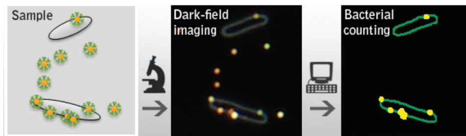
Figure 4. The antibody functionalized gold nanoparticles are used to image the E. coli directly based on the light-scattering of gold nanoparticles. Through this simple method, the E. coli can be easily counted. Reproduced with permission. [34] Copyright 2012, American Chemical Society.
